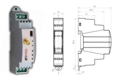
The receiver has an SMA connector for connecting an external ISM band antenna 868 MHz. Through the USB port it is possible to configure the receiver, especially in the ModBUS configuration, for customizing the mapping of the registers, in order to make available the information received from the wireless terminal devices.
